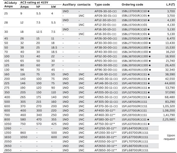
Complete the contactor type code by replacing \*\* with desired coil voltage, AF contactors have advanced electronic coil interface with wideband AC/DC coil
