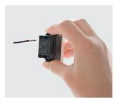
1. Strip the cable about 14 mm and introduce it into the terminal.
