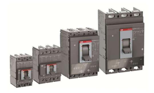
The new SACE FORMULA DSP family consists of four frames (P1, P2, P3 and P4) reaching up to 160A, 250A, 630A and 800A respectively. The four frames are available with thermal-magnetic trip units to cover the most common AC and DC fields. Availability of most requested accessories guarantees the possibility to fulfil the main applications needs.
