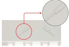
Visual signs provided in inner grids to guide proper fitment of easy installation and easy removal during fitment of mechanism with inner grid.
