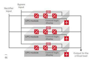
In DPA, each UPS module contains all the hardware and software required for full UPS system operation. Modules share no common components and each module is a fully functional UPS, so a DPA parallel system offers extremely high system reliability and uptime is maximized. UPS modules can be paralleled to provide redundancy or to increase the system's total capacity.
