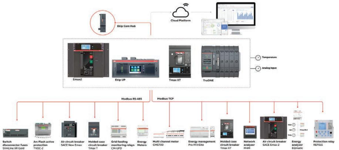
**External solution with ABB Ability™ Edge Industrial gateway**
