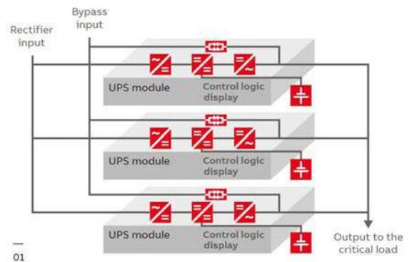
In DPA, each UPS module contains all the hardware and software required for full UPS system operation. Modules share no common components and each module is a fully functional UPS, so a DPA parallel system offers extremely high system reliability and uptime is maximized. UPS modules can be paralleled to provide redundancy or to increase the system's total capacity.
