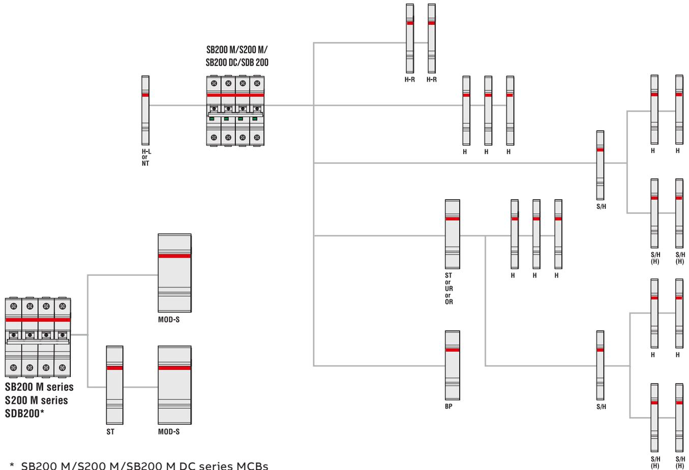
\* SB200 M/S200 M/SB200 M DC series MCBs and SDB200 switch disconnectors up to 3P or 2P+ST can be coupled with MOD-S
