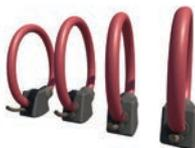
R4M Rogowski coils are flexible current transformer based on Rogowski technology, ideal to retrofit existing installations up to 12kA. Available in two different sizes (80mm or 200mm diameters), R4M coils are directly equipped with pre-wired removable terminals that perfectly fit M4M 20 Rogowski (3 Rogowski coil inputs) and M4M 30 Rogowski (4 Rogowski coil inputs), with no need for external integrators.
